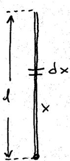
$$\int_{\text{asta}} r^2 dm = \int_0^l x^2 \lambda dx = \lambda \frac{l^3}{3} = \frac{m_a l^2}{3}$$
