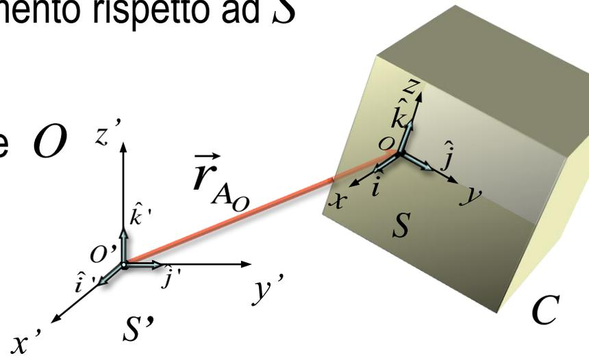
in generale :  $\vec{r}_{P_A} = \vec{r}_{P_R} + \vec{r}_{O_A}$      $\vec{v}_{P_A} = \cancel{\vec{v}_{P_R}} + \vec{v}_{O_A} + \vec{\omega}_A \times \vec{r}_{P_R}$
