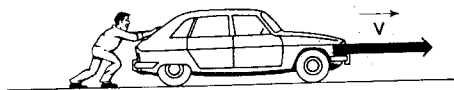
Figure A4. A breakdown: the action of the driver on the car is not larger than the reaction of the car on the driver
